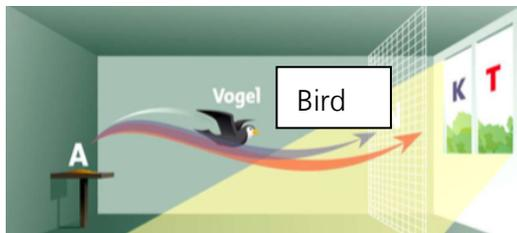
*During the approach test, a bird can either fly towards a control pane (K) or the Ornilux test pane (T). Tests are used to document which proportion of the birds flew towards the control pane and therefore recognised the Ornilux glass as an obstacle. The birds are stopped by a special net (N) well in advance of the panes, thus ensuring that they are not harmed during the test.*
